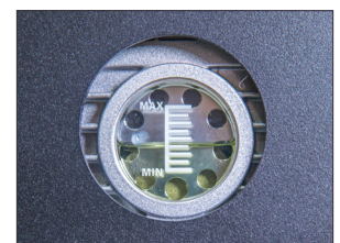
OIL LEVEL CHECK
