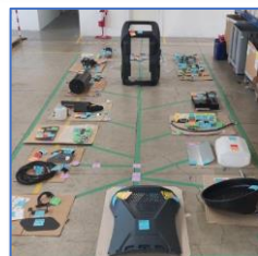
Fishbone: Root cause analysis by evaluation of each assembly component
