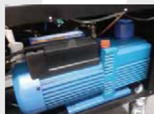
Strong Vacuum pump 142 l / min double stage
