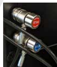
Quick couplers SAE J639 Hybrid function
